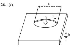
Shearing strain is created along the side surface of the punched disk. Note that the forces exerted on the disk are exerted along the circumference of the disk, and the total force exerted on its center only.
